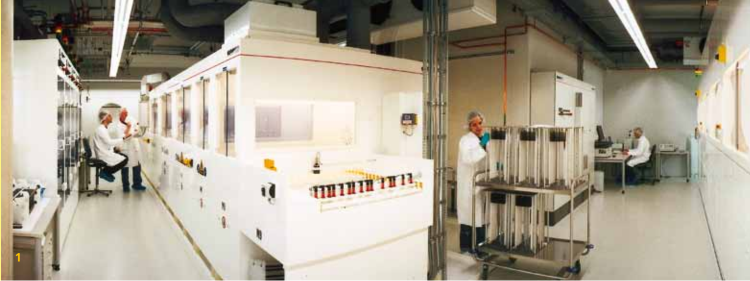
1 Wet-chemical processing equipment of the Photovoltaic Technology Evaluation Centre (PV-TEC) in Freiburg.
